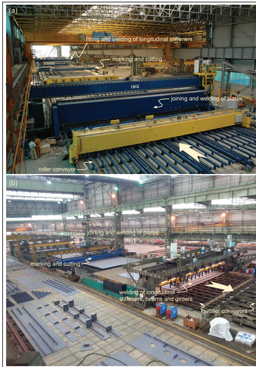
Figure 2. (a) Aerial view of the panel line at Fincantieri S.p.A. shipyard in Monfalcone showing the direction of panel flow from bottom to top (panels not present) and (b) aerial view of the panel line at Fincantieri S.p.A. shipyard in Ancona, with the panel flow moving from left to right.
