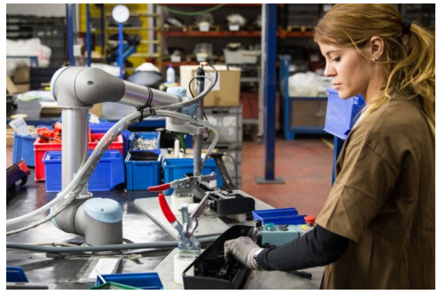
Fig. 1 Cobot-supported operator for a manual assembly task
