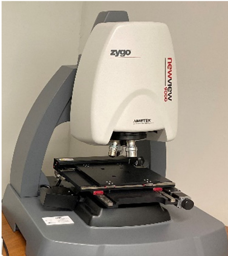
FIGURE 3 The Coherence Scanning Interferometre, Zygo NewView 9000, exploited to perform the measurements
